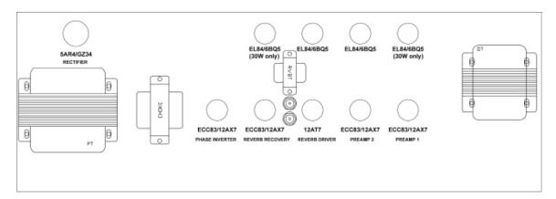
The Invader uses four ECC83/12AX7 tubes, one ECC81/12AT7 tube, and two 6BQ5/EL84 output tubes (four EL84s in the 30W version). It also uses a single 5AR4/GZ34 rectifier tube.
